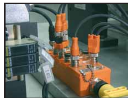
Module depicted with M12" bus connection and on-board 7/8" power auxiliary power connection with T-Connector.
